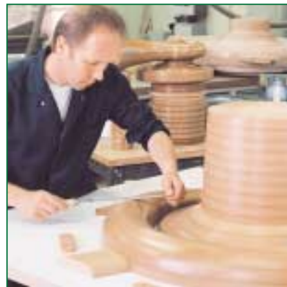
Hand-crafted: a patternmaker at ENSIVAL puts the final touches to a new centrifugal pump design
